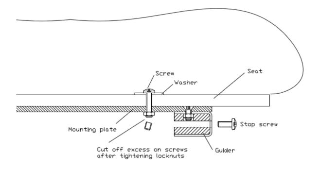
**9. Stop-screw in.** From underneath the seat; turn the guiders' stop-screw(J) all the way in, without using force.
