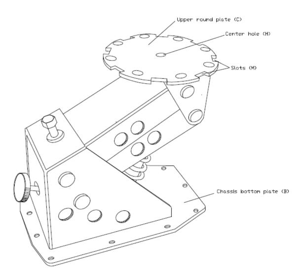
**6. Fix turning plate onto the chassis.** To do this; compress the turning plate's(D) spring by turning the lever(E) and fit the (now lifted) plastic stopper(F) into one of the eight(8) slots(M) on the upper, round plate(C).
