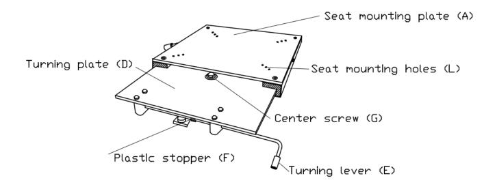
**4. Attach plate under seat**. Fasten the seat mounting plate(A) under the seat with the accompanying screws & nuts (if provided) – or other, if they don't fit your specific seat.
