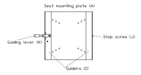
**3. Slide plates apart.** Remove the turning plate (D) from the guiders(I) on the seat mounting plate(A). You need to engage the guider lever(K) to release the turning plate(D).
