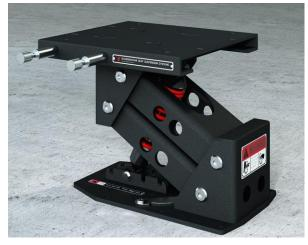
Height: 295-330mm / 11,5-13" Swivel included: 360° in 8 lock positions Slide included: fore/aft: 120mm / 5" Adjustable pre-load: 50-130kg / 110-285lb Weight: 12,5kg / 27lb Deck mount: 375x225mm / 14,5x9" Seat mount: 330x315mm / 13x12,5" (Handles 250mm / 10" from center-line)
