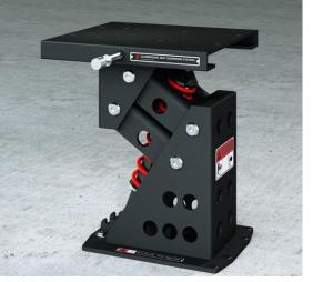
Height: 385-430mm / 15-17" Slide included: fore/aft: 120mm / 5" Adjustable pre-load: 50-130kg / 110-285lb Weight: 13kg / 28lb Various deck mount size/shape available. Seat mount: 330x315mm / 13x12,5" (Handle 250mm / 10" from center-line)
