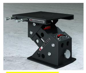
Height: 305mm / 12" Swivel included: 360° in 8 lock positions Slide included: fore/aft: 120mm / 5" Adjustable pre-load: 50-130kg / 110-285lb Weight: 14kg / 31lb Various deck mount size/shape available. Seat mount: 330x315mm / 13x12,5" (Handles 250mm / 10" from center-line)
