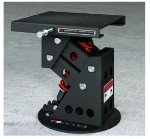
Height: 335-370mm / 13-14,5" Slide included: fore/aft: 120mm / 5" Adjustable pre-load: 50-130kg / 110-285lb Weight: 12kg / 26lb Various deck mount size/shape available. Seat mount: 330x315mm / 13x12,5" (Handle 250mm / 10" from center-line)
