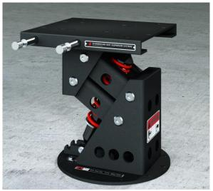
Height: 345-380mm / 13,5-15" Swivel included: 360° in 8 lock positions Slide included: fore/aft: 120mm / 5" Adjustable pre-load: 50-130kg / 110-285lb Weight: 14kg / 31lb Various deck mount size/shape available. Seat mount: 330x315mm / 13x12,5"
