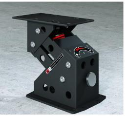
Height: 325mm / 13" Adjustable pre-load: 50-130kg / 110-285lb Weight: 11kg / 24b Various deck mount size/shape available. Seat mount: 330x180mm / 13x7"
