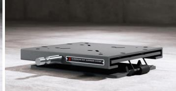
Height: 95mm / 4" Swivel included: 360° in 8 lock positions Slide included: fore/aft: 120mm / 5" Weight: 8,5kg / 19lb Adjustable for weights: 50-130kg / 110-285lb Deck mount: 330x230mm/13x9" Seat mount: 330x315mm/13x12,5" (Handles 250mm / 10" from center-line)
