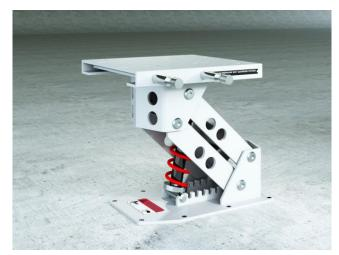
Height: 355mm / 14" Swivel included: 360° in 8 lock positions Slide included: fore/aft: 120mm / 5" Adjustable pre-load: 50-130kg / 110-285lb Weight: 12kg / 26lb Various deck mount size/shape available. Seat mount: 330x315mm / 13x12,5" (Handles 250mm / 10" from center-line)
