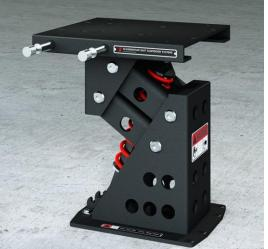
Height: 395-440mm / 15,5-17,5" Swivel included: 360° in 8 lock positions Slide included: fore/aft: 120mm / 5" Adjustable pre-load: 50-130kg / 110-285lb Weight: 15kg / 33lb Various deck mount size/shape available. Seat mount: 330x315mm / 13x12,5" (Handles 250mm / 10" from center-line)
