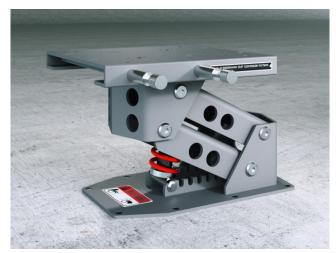
Height: 260mm / 10,5" Swivel included: 360° in 8 lock positions Slide included: fore/aft: 120mm / 5" Adjustable pre-load: 50-130kg / 110-285lb Weight: 11kg / 24lb Various deck mount size/shape available. Seat mount: 330x315mm / 13x12,5" (Handles 250mm / 10" from center-line)
