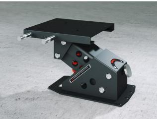
Height: 275mm / 11" Swivel included: 360° in 8 lock positions Slide included: fore/aft: 120mm / 5" Adjustable pre-load: 50-130kg / 110-285lb Weight: 13,5kg / 30lb Various deck mount size/shape available. Seat mount: 330x315mm / 13x12,5" (Handles 250mm / 10" from center-line)
