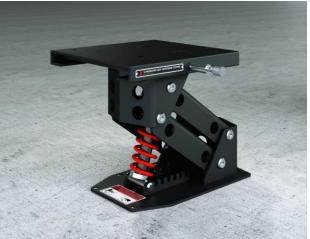
Height: 305mm / 12" Slide included: fore/aft: 120mm / 5" Adjustable pre-load: 50-130kg / 110-285lb Weight: 10kg / 22lb Various deck mount size/shape available. Seat mount: 330x315mm / 13x12,5" (Handle 250mm / 10" from center-line)
