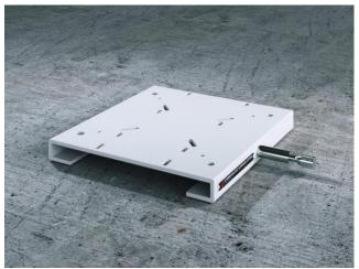
Height: 39mm / 1,5" Slide included: fore/aft: 120mm / 5" Weight: 4,5kg / 10lb Deck mount: Ø190mm / 7,5" Deck mount holes: Ø160mm / 6" Seat mount: 330x315mm / 13x12,5" (Handle 250mm / 10" from center-line)
