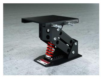
Height: 315mm / 12,5" Swivel included: 360° in 8 lock positions Slide included: fore/aft: 120mm / 5" Adjustable pre-load: 50-130kg / 110-285lb Weight: 12kg / 26lb Various deck mount size/shape available. Seat mount: 330x315mm / 13x12,5" (Handles 250mm / 10" from center-line)
