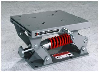
Height: 190mm / 7,5" Slide included: fore/aft: 120mm / 5" Adjustable pre-load: 50-130kg / 110-285lb Weight: 11,5kg / 25lb Deck mount: 330x230mm / 13x9" Seat mount: 330x315mm / 13x12,5" (Handle 250mm / 10" from center-line)
