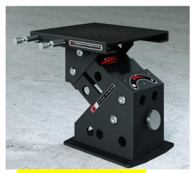
Height: 350mm / 14" Swivel included: 360° in 8 lock positions Slide included: fore/aft: 120mm / 5" Adjustable pre-load: 50-130kg / 110-285lb Weight: 15kg / 33lb Various deck mount size/shape available. Seat mount: 330x315mm / 13x12,5" (Handles 250mm / 10" from center-line)
