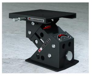
Height: 295mm / 11,5" Slide included: fore/aft: 120mm / 5" Adjustable pre-load: 50-130kg / 110-285lb Weight: 12,5kg / 28lb Various deck mount size/shape available. Seat mount: 330x315mm / 13x12,5" (Handle 250mm / 10" from center-line)
