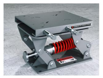
Height: 220mm / 8,5" Swivel included: 360° in 8 lock positions Slide included: fore/aft: 120mm / 5" Adjustable pre-load: 50-130kg / 110-285lb Weight: 13kg / 28lb Deck mount: 330x230mm / 13x9" Seat mount: 330x315mm / 13x12,5" (Handles 250mm / 10" from center-line)
