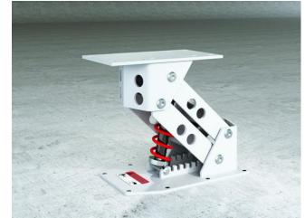
Height: 330mm / 13" Adjustable pre-load: 50-130kg / 110-285lb Weight: 8kg / 18lb Various deck mount size/shape available. Seat mount: 330x185mm / 13x7"
