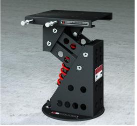
Height: 445-485mm / 17,5-19,5" Swivel included: 360° in 8 lock positions Slide included: fore/aft: 120mm / 5" Adjustable pre-load: 50-130kg / 110-285lb Weight: 16kg / 35lb Various deck mount size/shape available. Seat mount: 330x315mm / 13x12,5" (Handles 250mm / 10" from center-line)
