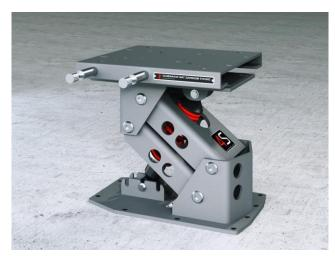
Height: 295-330mm / 11,5-13" Swivel included: 360° in 8 positions Slide included: fore/aft: 120mm / 5" Adjustable pre-load: 50-130kg / 110-285lb Weight: 13kg / 29lb Deck mount: 375x225mm / 14,5x9" Seat mount: 330x315mm / 13x12,5" (Handles 250mm / 10" from center-line)
